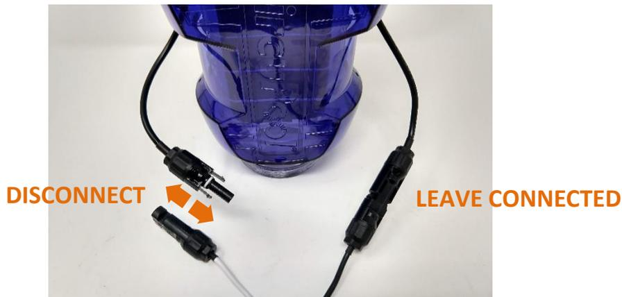
**IMPORTANT:** the next step will determine the second part of the System Error 2 code. Once determined, power the Control Module back off as soon as possible and restore the normal cable connection. **Do not leave the connections connected to only one side and powered for too long, as it could damage the internal power supply.**
