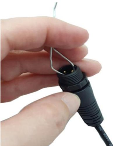
1. Disconnect the Temperature Sensor cable connection.
