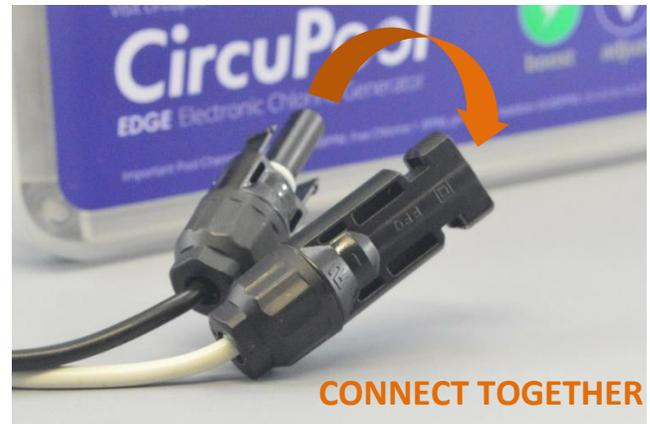
**IMPORTANT:** the next step will determine the second part of the System Error 1 code. Once determined, power the Control Module back off as soon as possible and disconnect the above cable connection. **Do not leave the connections to power supply together for too long, as it could damage the internal power supply.**
