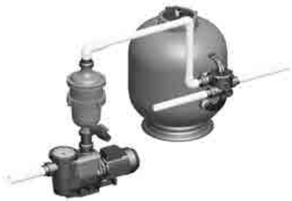
Typical Installation with a Sand Filter
